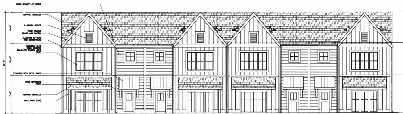
elev 5 FRONT ELEVATION 1/8"=1'-0" A201 FOUR UNIT BLDG
